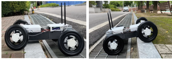
(c) Height less than 117.5mm (d) Height over 117.5mm Fig. 15. Experiment to Overcome Steps
